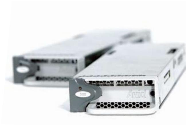
Each intelligent Avid ISIS Storage Blade is a mini server including disks, processor, memory, and networking. The storage blades communicate with one another, constantly balance loads, and redistribute data in the case of drive failure.
